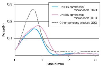
\* Measured by puncturing PA film at 90° with a load cell of 10N at a test speed of 200mm/min.
